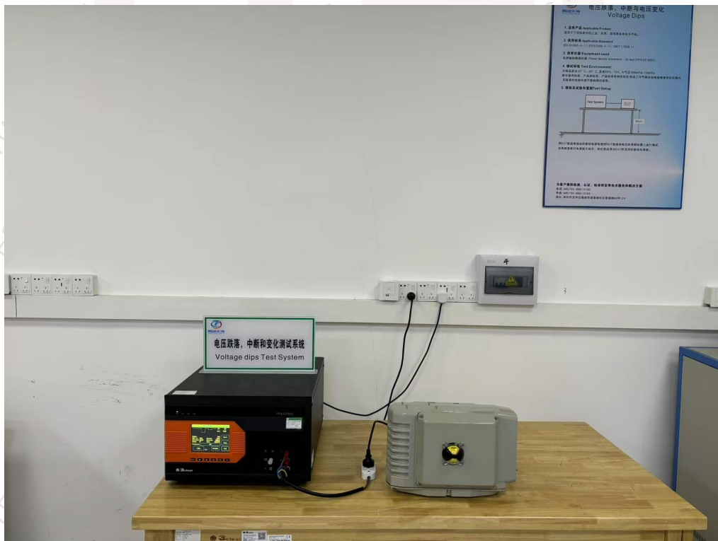
Photograph 10: Setup for Voltage Dips And Interruptions
