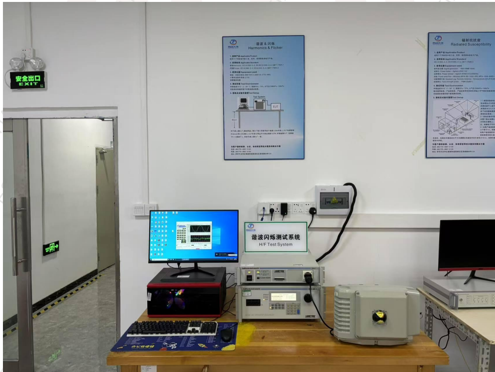
Photograph 4: Setup for Voltage Fluctuation and Flicker
