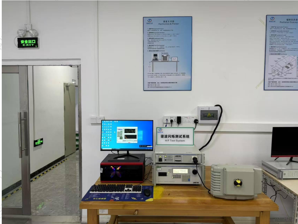
Photograph 3: Setup for Harmonic Current Emission
