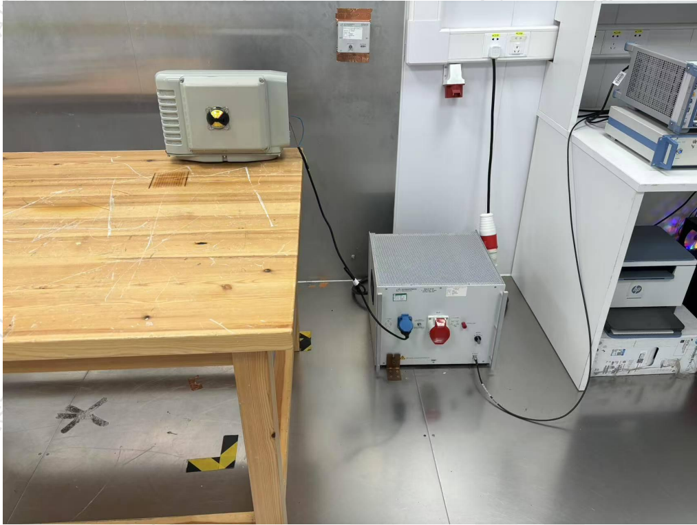
Photograph 2: Setup for Radiated Emission
